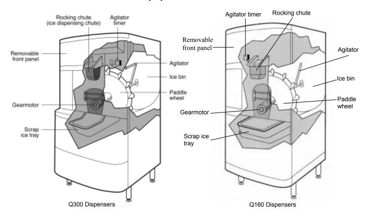
The operation of the Q Series ice dispenser can be divided into three main operations. They are Dispenser Activation, Ice Pick-Up and Ice Delivery.
